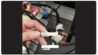
12. Thread both blower wires through the hood body wiring holes. Connect the 9-pin blower plugs and black single pin power cables together from both blowers.
