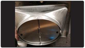
Attach 10" round blower collar on top of the hood body by (4) M4x8 screws.
