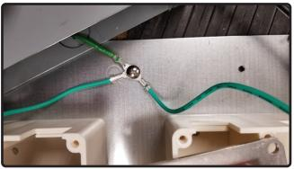
16. Secure the (3) ground wires together by (1) screw. The ground wires are from the electrical box and each control board.
