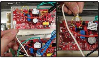
14. Locate loose white power wire with female spade connector from the main control board and attach it to the PBD-1300B control board.
