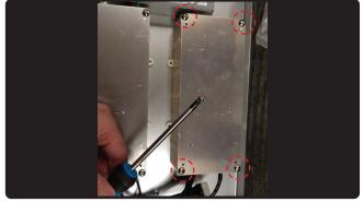
17. Secure both control boards back to the component box by (4) screws each.
