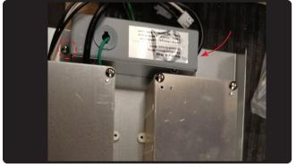
18. Secure the electrical box by (2) screws.
