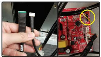
15. Connect the 5-pin white male connector from PBD-1300B control board to the 5-pin female connector leading from the range hood's switch assembly. Do <u>not</u> connect the 5-pin female connector to the PBD-1300B control board.
